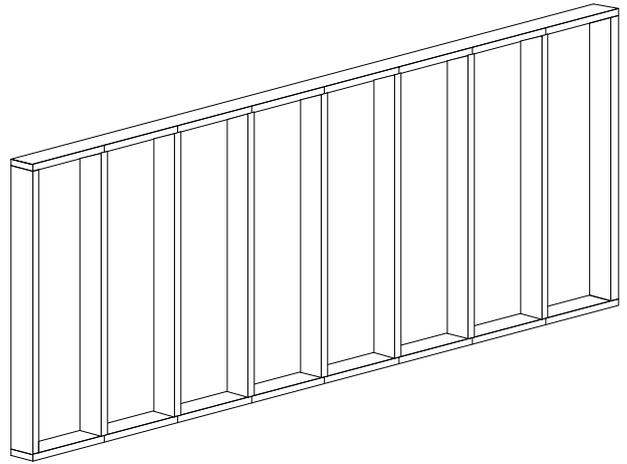
NB: Whereas 'stick-building' entails cutting and fitting diagonal 'bracing' timbers after erection to keep the open framework squared up; our method is to simply nail sheets of plywood or OSB onto the upper face of the open-framing ~ the 'sheathing' then acts like a giant 'gusset-plate' and keeps the whole panel truly rectangular during erection and carrying the subsequent structural loadings!
