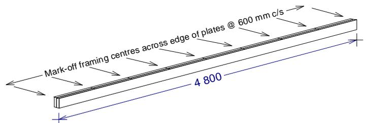
Assuming a simple 4.8 m (16 ft.) long wall-panel; our example will need nine (identical) vertical framing members ~ so simply mark off the required length as per the 'cutting schedule' (using a steel tape-measure) and cut the nine timbers to length.
